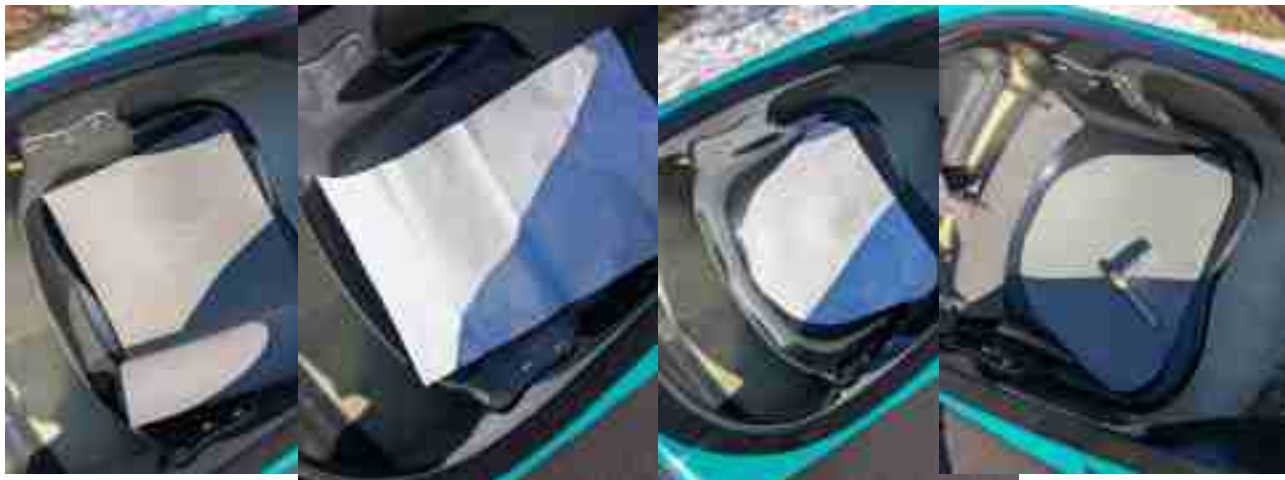
Cutting and installing foam pad: Roll of 1/4" closed cell foam, heavy paper for pattern, pattern traced and cut, pad cut but not glued. Note foam for seat bottom back cut but not glued.
