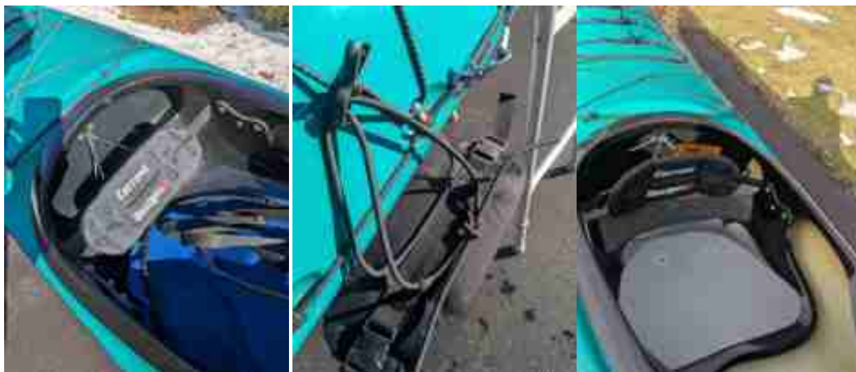
Loose bungee on back band; Detail of bungee support for back band; Installed seat with pads, properly supported back band and "If found..." sticker.
