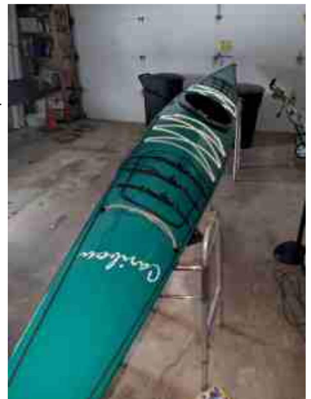
Flash photo of completed bungee and paddle park reveals Night-ize reflective property of bungee.
