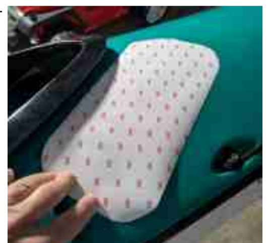
3M paint protection film being fitted. The backing peels off and you spray a water-soap slip fluid to position the film and squeegee out air bubbles.
