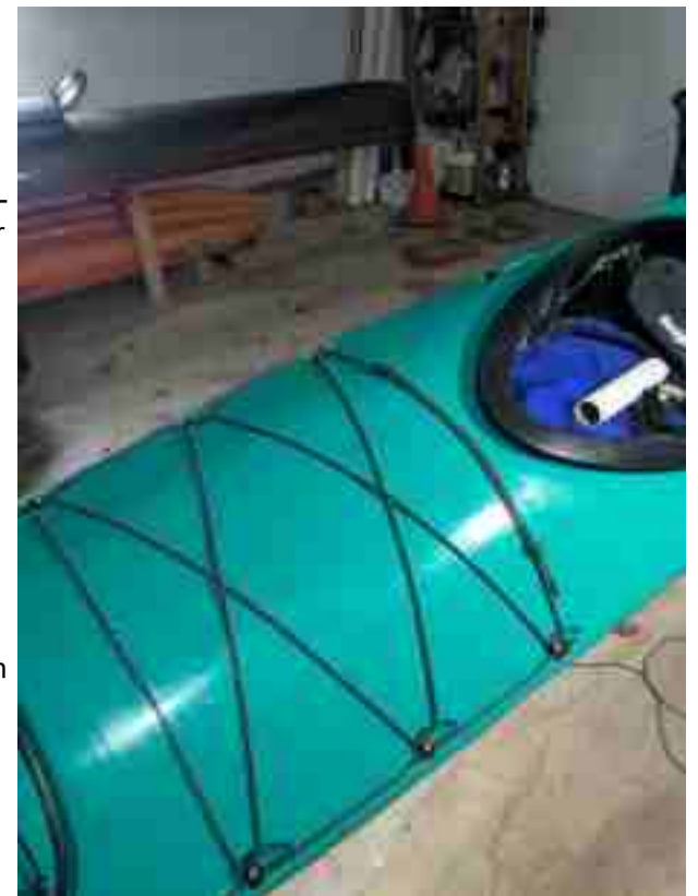
Fore deck bungee pattern complete with grapevine knot
