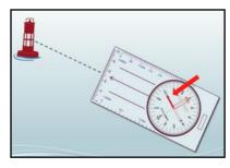
Know how to take a bearing. Identify an object to use for your bearing. Point your compass at that object. Identify the needle that points to magnetic north.
