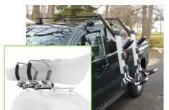
The most expensive method, but the easiest for one person, is the load-assist saddle system. These rack systems attach to the vehicle or rack system cross bars. They unlatch and swing down from the side of the vehicle so that the cradles are about waist high and vertically oriented. The kayak is simply placed onto the cradles on its side, strapped down, and then, with a spring assist, swung back onto the roof of the vehicle with the kayak ending up upright like a standard pair of saddles.
