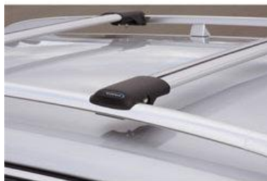
Pictured, Yakima's new Whisbar ® installed on a factory rail. A marked improvement over the round bars. Thule has countered with a similar Aeroblade ® system. Both are designed to reduce wind noise. They are more expensive than the older rack systems. I suspect that the older systems will be eventually phased out. These are not compatible with some of the older style rack system's components.
