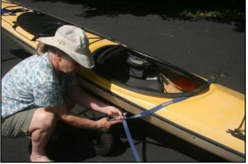
Pass the strap around the front frame member, and cut the excess about 2" beyond it, about where Sue has her right index finger. Use a match or lighter to heat seal the cut ends to prevent fraying. Next, making a loop which will fit around the cart frame, use an awl or other sharp implement to make a ¼" hole through the straps. Be sure to make to loop big enough.
