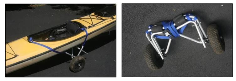
Secure both straps firmly around the cockpit rim, front and back. With this method, much faster than using one long strap, the cart cannot collapse or twist. The cart will stay firmly attached if the kayak has to be carried for a short stretch or even if it tips over.
