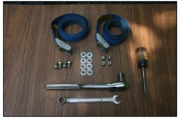
They consist of two straps, four ¼"-20 x ½" hex nuts, the corresponding four nylon insert lock nuts, and eight flat washers. The fasteners should all be 316 stainless steel, which you can find at West Marine and other boating supply stores. Most regular hardware stores stock fasteners of 304 stainless steel, which while fairly corrosion resistant and less expensive, is not rated for salt water. You will also need some tools to tighten the nuts and bolts, and finally an awl.
