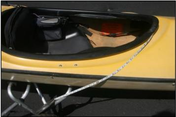
The next step is to take the buckle end and run it from the top of the front frame member to a bit past the center line of the kayak in front of the cockpit rim.
