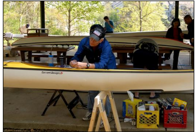
David Wilson Replacing Deck Lines photo by DJ Manalo
